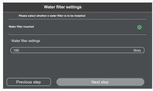
A water filter is necessary with a water hardness higher than 5 °dKH to prevent damage to the coffee machine. The water filter must be changed regularly.
