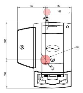
disposal (2) and drain hose (1) on bottom of machine (minimum distance (A) of hole from machine: 40 mm).
