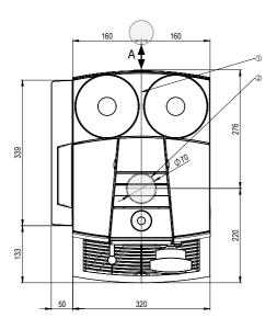
Figure: Position of tube section for coffee grounds disposal (2) and drain hose (1) on bottom of machine (minimum distance (A) of hole from machine: 40 mm).
